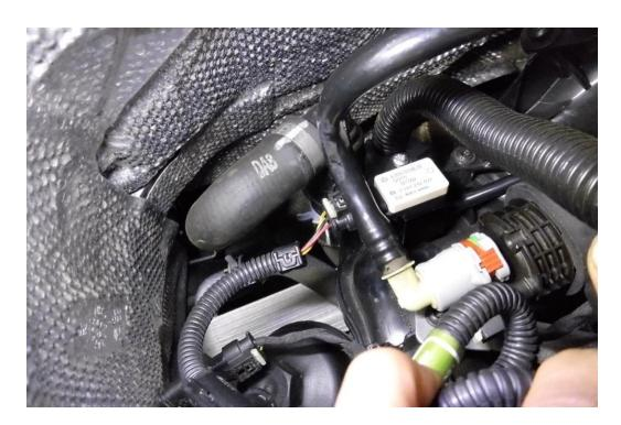
7. Run the silicon hosing along with the black vacuum pipe and use the cable ties provided to attach it.
