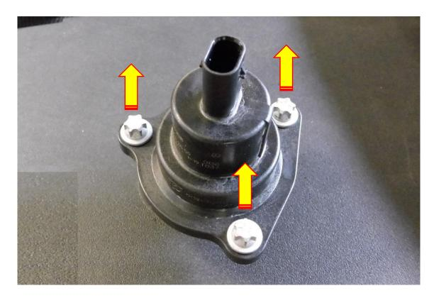
Locate the map sensor attached to the inlet manifold and unplug the wiring loom going to it. The sensor is held in place with a T25 Torx fastener, use the relevant Torx driver to remove it, the sensor will now pull out of the inlet manifold.
