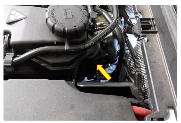
3. Disconnect the wiring loom going to the valve. Slide the white locking tab back then fully depress the clip which will allow the plug to be removed.
