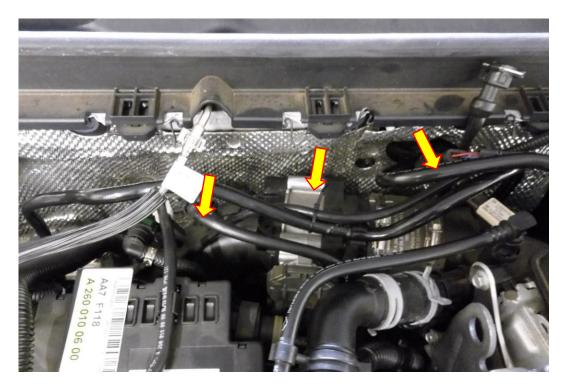
8. Fit the Forge replacement valve where the old valve was situated, secure it in place using the supplied M6x16 Allen cap head fasteners. Use a 5mm Allen key to do this. The orientation of the valve should be that the base boost port is pointing downwards.
