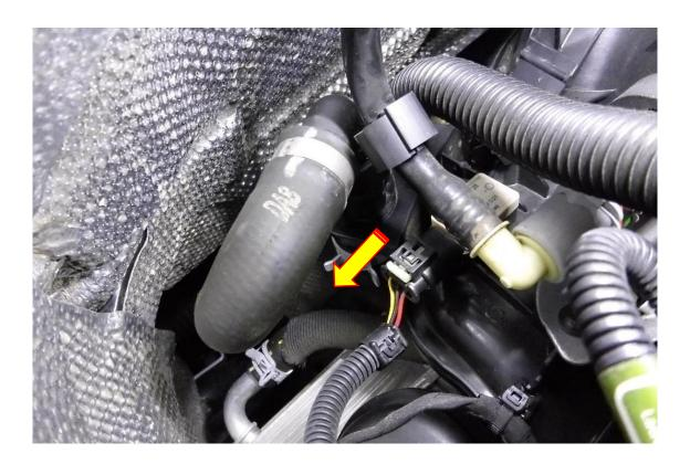
6. Take the removed sensor and fit it to the machined vacuum boss as shown in the picture below. Attach the supplied silicon hose to the vac port on the boss then re fit both attached items onto the manifold using the M6x40 fastener in the FMDV26 kit, secure the sensor and boss with a pozi drive. Plug the wiring loom back into the sensor.
