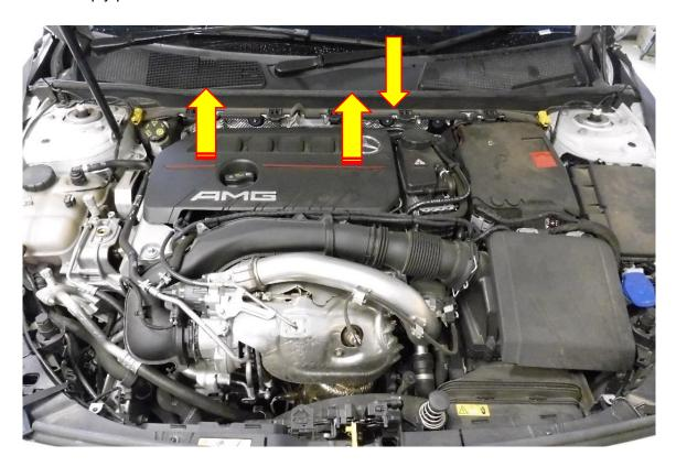
2. Locate the valve, it is situated on the back of the charge cooler which itself is located next to the vehicles battery.
